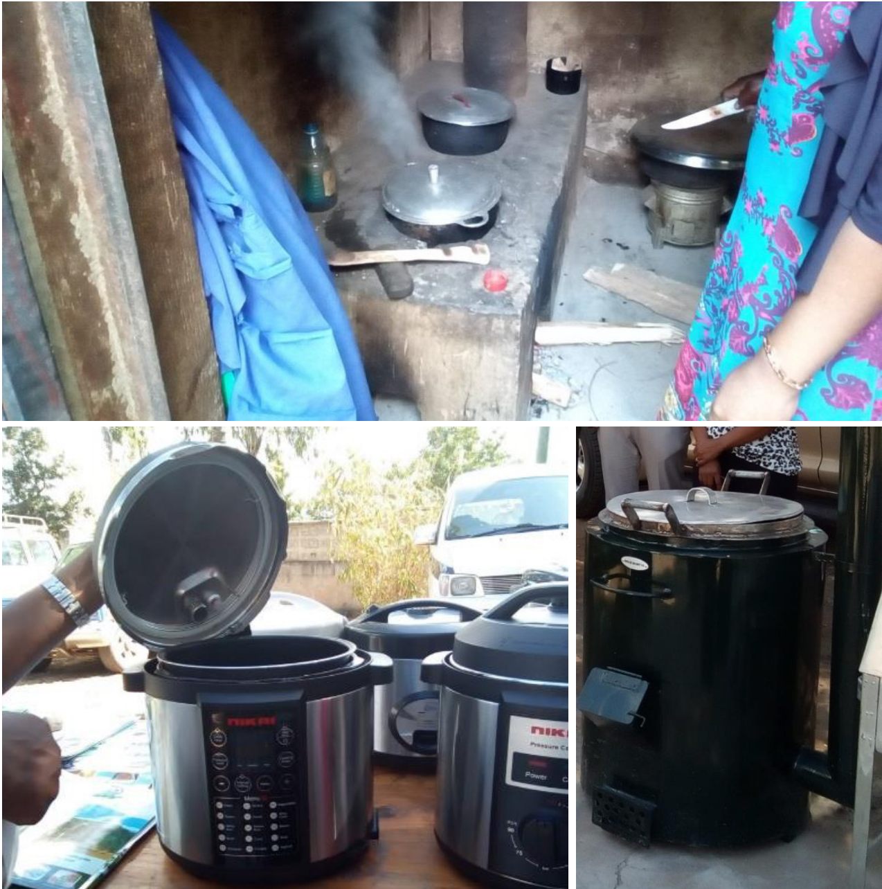
Figure 7: Future cooking options: Improved Cookstove (ICS), high efficiency improved cookstove, high-efficient electric pressure cooker
