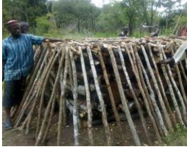
An Improved Basic Earth Mound Kiln (IBEK) (Photo: TaTEDO)
